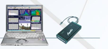
The new SINUS **Apollo** box is our flexible and inexpensive 4-channel front-end device with USB 2.0 interface. The robust and small box can easily be used with any Windows Personal Computer and a wide range of application software.
